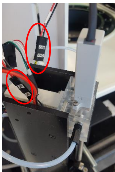
Fig. 2.21: Disconnecting Dilutor Electrovalve
